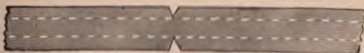
Fig. 164—Plain Bar with Four Bars Welded Upon It, Leaving Gaps at Center.
