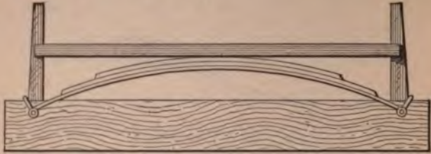
A Spring for Farm Wagons. Fig. 181—Showing Spring in Position.
