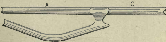
FIG. 153.—SHOWING HOW THE PIECES ARE JOINED AND WELDED IN MAKING AN OFFSET.
