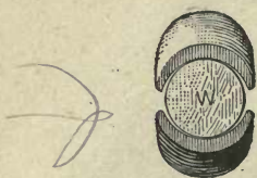
FIG. 142.—SHAPE OF TONG JAWS FOR ROUND WORK.
