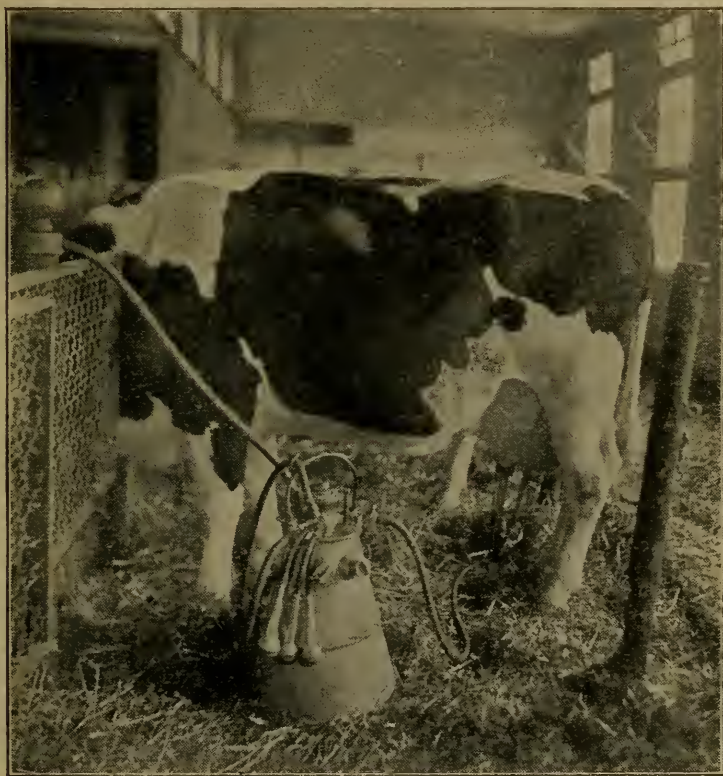
X.—MILKING MACHINE PAIL with one set of teat cups in operation. The pail is divided by a partition which keeps the milk of two cows separately.
